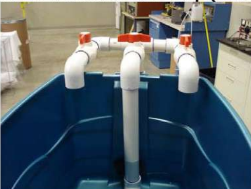
Inlet Manifolds from Pump (with Ball Valves)
