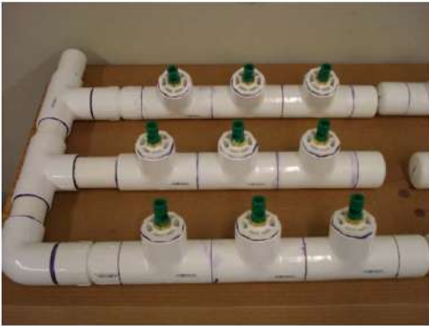
Side manifolds with mini educators installed
