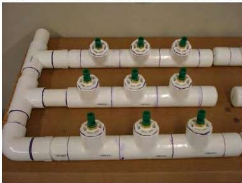
Side manifolds with mini educators installed
